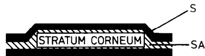
Fig. 1. Stratum corneum–silicone membrane sandwich (see text). S, silicone membrane; SA, silicone adhesive.
